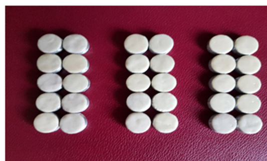
Fig 2: Samples after Opaque and dentin ceramic application
