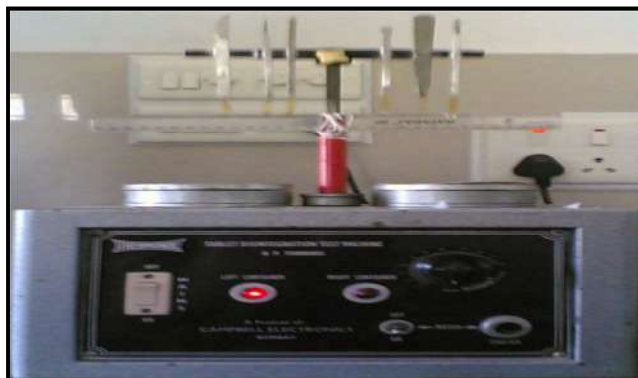
Fig.3 Modified Folding Endurance Tester
