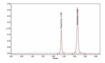
The retention times were 2.368 min and 3.129 min for Theophylline and Etophylline respectively. These retention times did not vary to any considerable degree during and in between analyses (% R.S.D. less than 2% for the retention time of each peak). System suitability test are the
