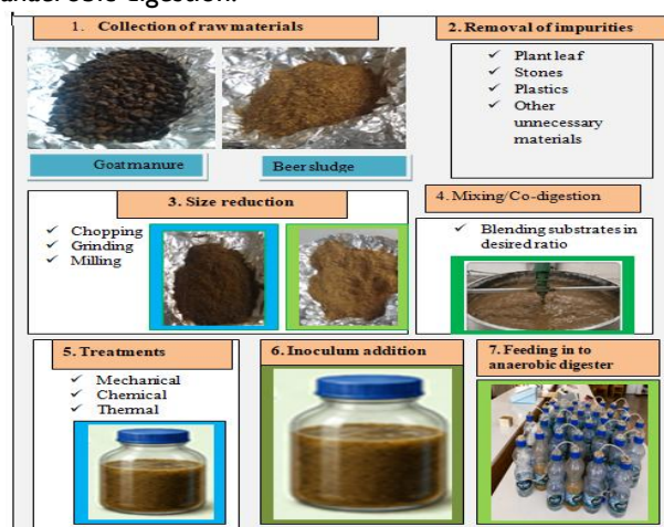
Figure 01: Highlights of the anaerobic digestion configuration and experimental process at the laboratory scale
