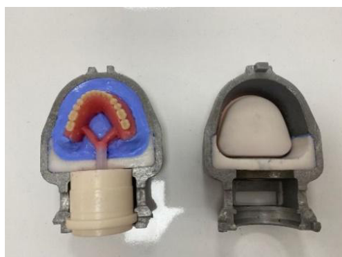
Fig. 8 Wax Channels in SR IVOCAP Flasks
