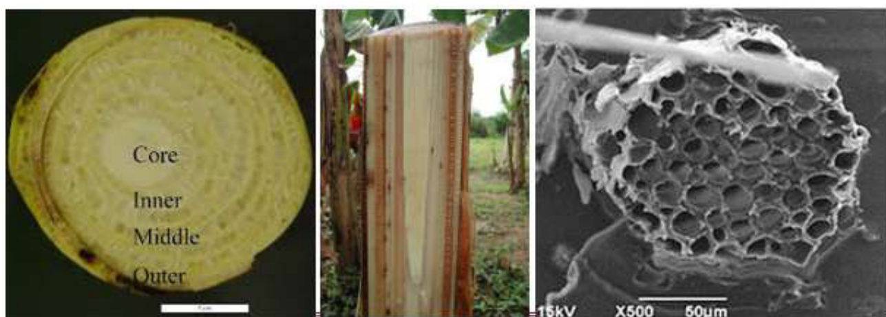
Fig. 3. Pseudostem structure of banana 28 ; (a) transverse section, (b) cross-sectional view, and (c) bundles of pseudostem fibres
